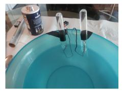
Step 4: Touch the other end of the copper wire to the ends of a 9 volt battery. You can try it with a loop as shown.
